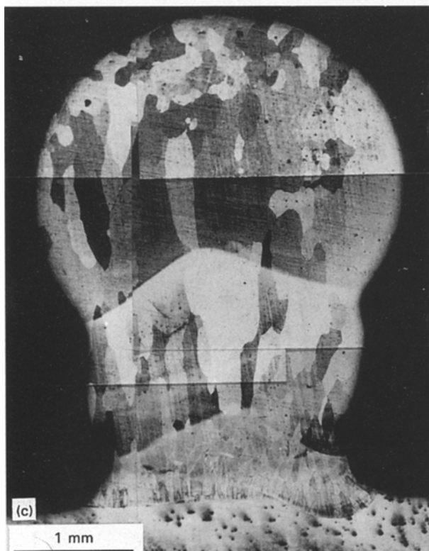
Figure 4 Optical macrographs of transverse sections of functionally graded Fe–Al coatings produced at 1.8 kW, 3 mm, 7 \text{ mm s}^{-1} and 0.183 \text{ g s}^{-1} Fe and various Al powder flow rates ( 0.032 to 0.1 \text{ g s}^{-1} ); (a) single layer; (b) two-layer FG coating; (c) three-layer FG coatings.
